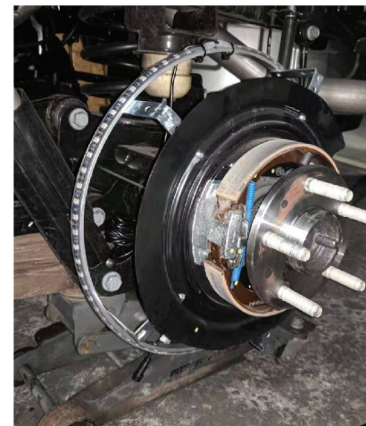
90 Deg brackets are mounted on backside of the dust shield
